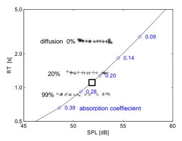
Figure 6: RT and SPL values from a ray-tracing computer model for three different diffusion factors. Room size is 21  $^{-}12 ^{-}5.5 \text{ m}^{3}$ ;  $\mathbf{a} = 0.25$  (small square). There is one source position and 20 microphone positions.
