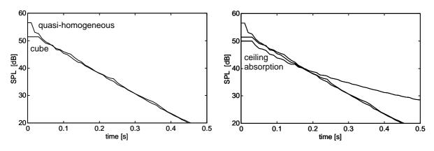
Figure 2: Decay curves when a cubic space with homogeneous absorption is compared with a rectangle with non-homogeneous absorption. See text for explanation.
