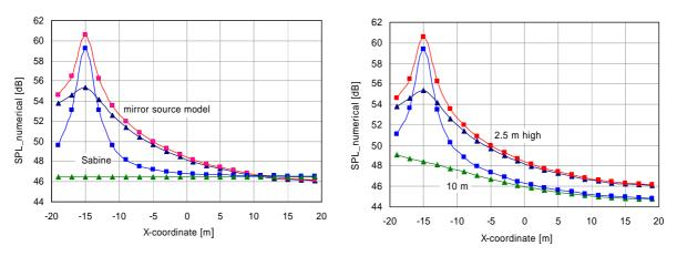
Figure 4: Calculations for a room with x and y coordinates ranging from -20 to +20 m. Source position is at (-15, -15), the microphone is at y = -14, while x-values range from -19 to +19; so the shortest distance is 1 m and since  $L_W = 70$ , SPL is predicted by common theory as 59.0 dB. All surfaces have the same absorption coefficient of 20%.
