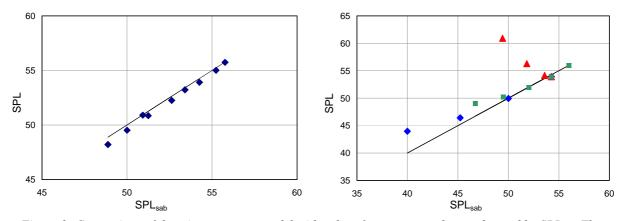
Figure 3: Comparison of the mirror sources model with values from common theory, denoted by SPL<sub>sab</sub>. The source power level is taken as 70 dB (re 10-<sup>12</sup> W). In the left figure all spaces are cubic (10<sup>-10</sup> 10 m<sup>3</sup>). The basis is the (54.3, 53.9) value where all surfaces have the same absorption coefficient of 20%. Other dots represent a variety of absorption coefficients with 20 / 20 / 99% as an extreme case.
